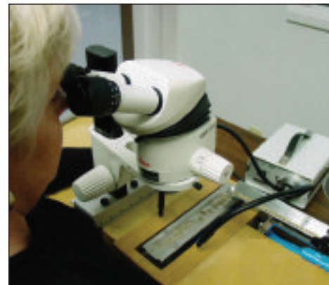
The ergo-vision testing station uses a small vibratory to steadily move seeds into the analyst's field of vision.
